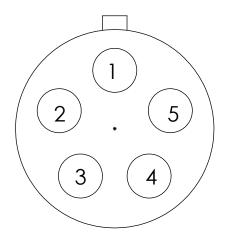
This Diagram to be used for wiring 5 way connector.
