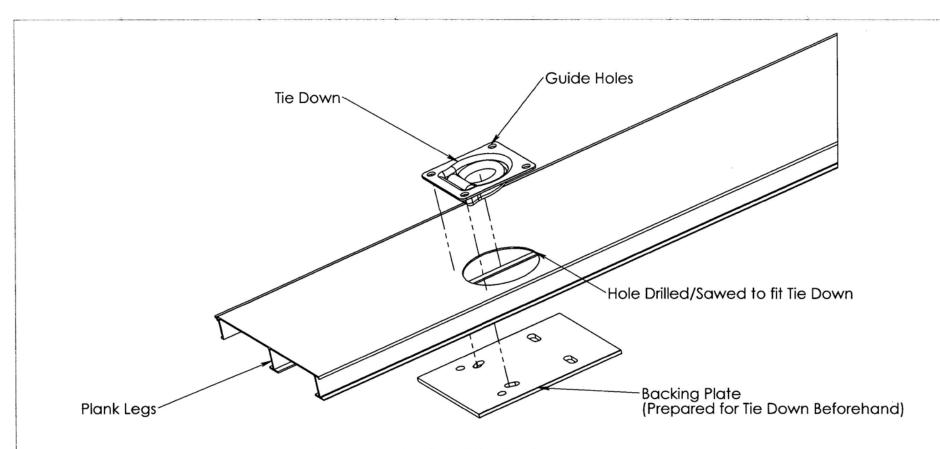
First Drill a hole in the plank in the location you want to install the tie down.
