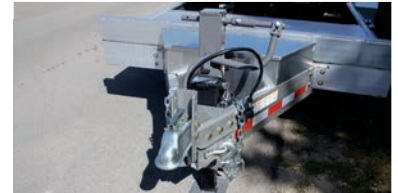
42" Long A-Frame Aluminum Tongue w/ 2 5/16" Adjustable Coupler
