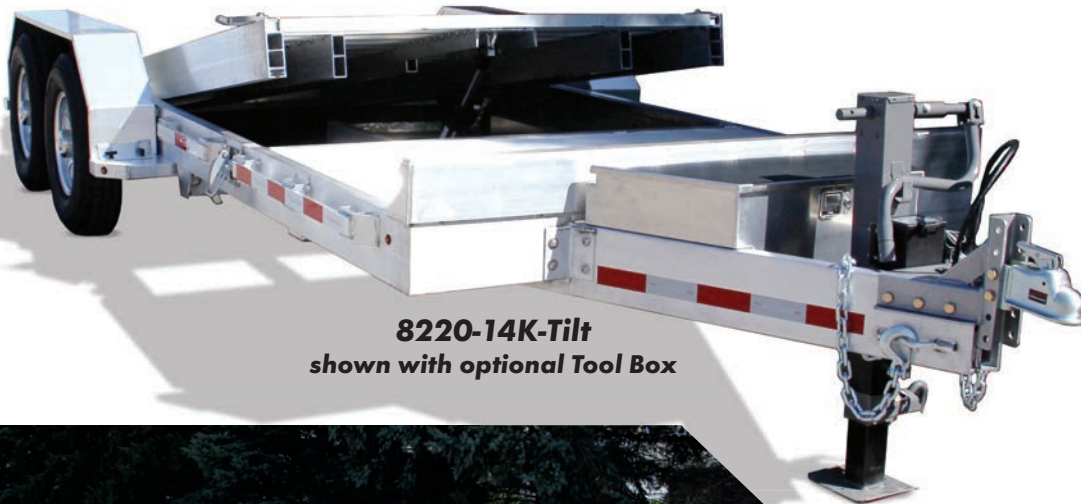
42" Long A-Frame Aluminum Tongue w/ 2 5/16" Adjustable Coupler
