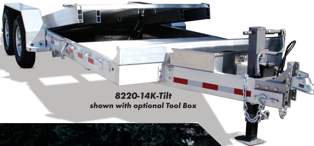
42" Long A-Frame Aluminum Tongue w/ 2 5/16" Adjustable Coupler
