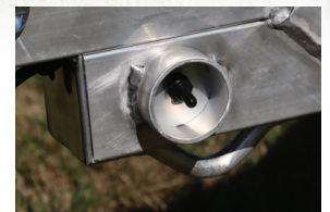
Light Switch for Bed Lights
