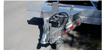
42" Long A-Frame Aluminum Tongue w/ 2 5/16" Adjustable Coupler
